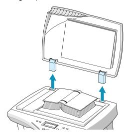
To insert the cover in place, hold it as shown and insert its hinges into the holes. Then close the top cover.
